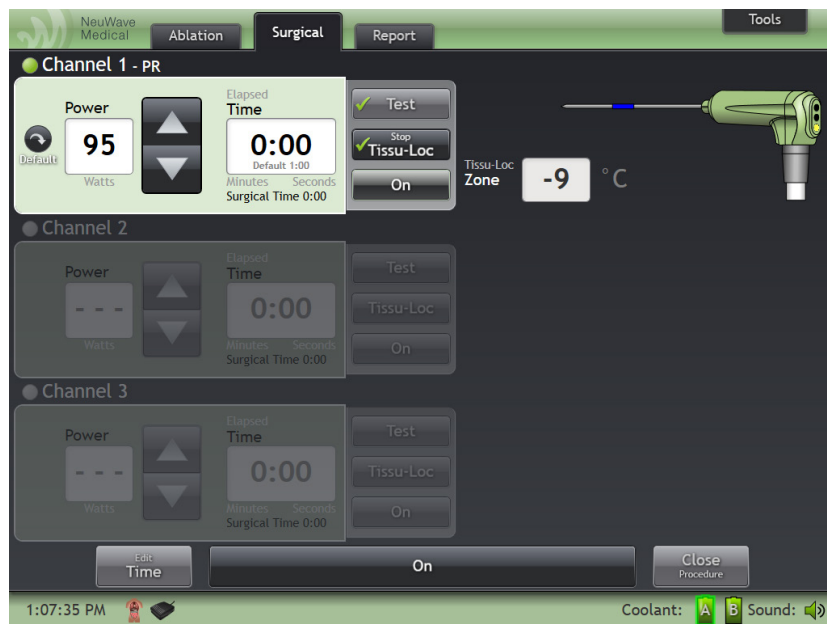
Figure 4-24: A NEUWAVE PR Probe is connected to Channel 1 and the Tissue-Loc button is enabled and active.
