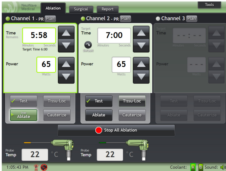
Figure 4-17: Channel 1 Ablate Button has been pressed.
