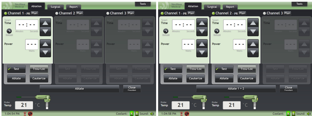
Figure 4-12: Ablation Tab with one probe connected (left) and with two probes connected (right)
