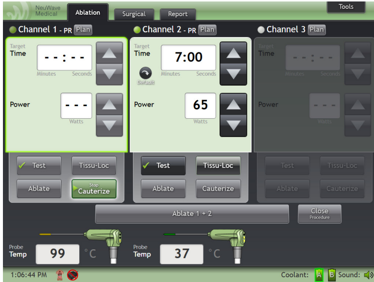
Figure 4-20: Ablation Tab with Cauterize Button in use for Channel 1 probe.
