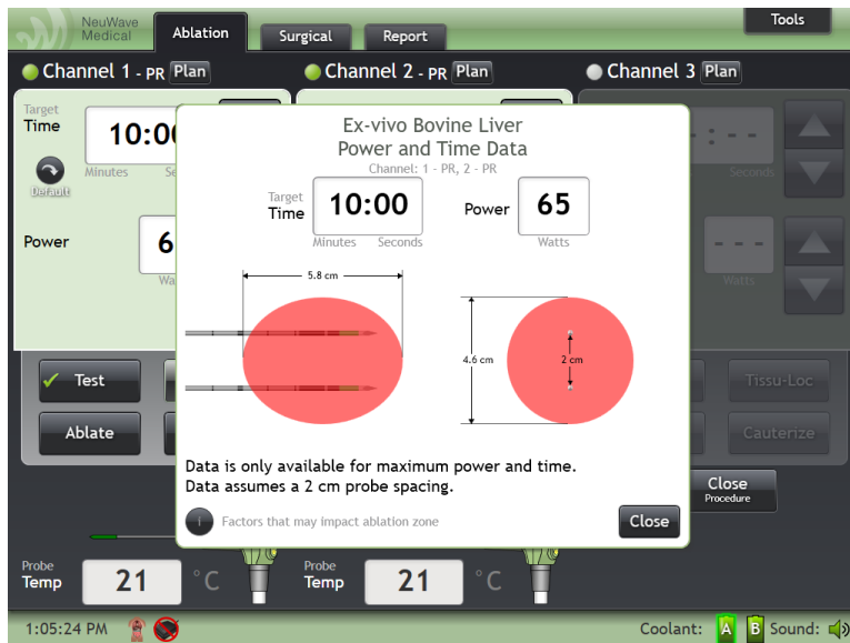
Figure 3-24: Example of Ablation Visualization Window for a multiple probe ablation
