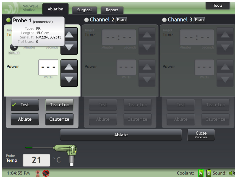
Figure 4-13: Touch the Channel Number to see probe identification information.
