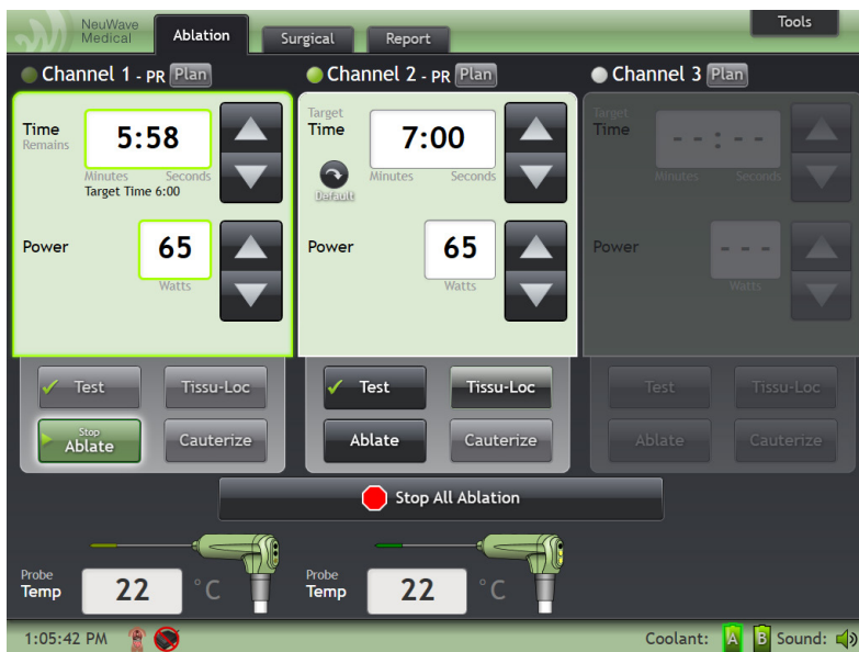
Figure 4-19: Channel 1 probe ablating and Channel 2 probe ready for use but not delivering energy.
