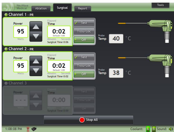
Figure 4-27: Surgical Tab showing Off/Stop controls.
