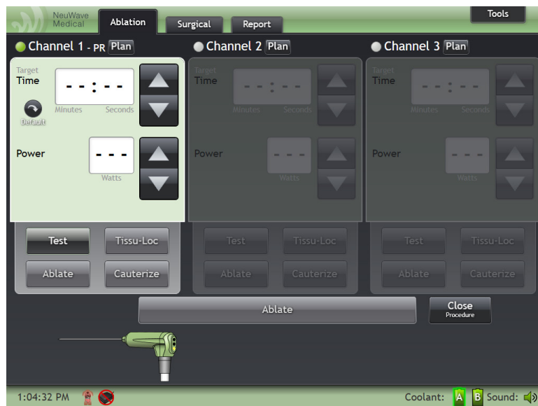
Figure 4-7: Ablation Tab After Channel 1 Probe connected to PDM.
