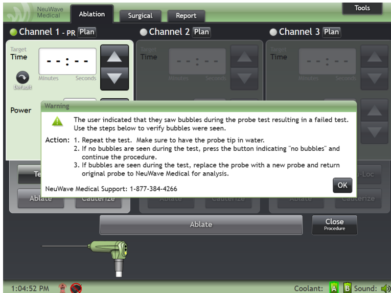
Figure 4-10: When the bottle icon with bubbles is selected, a 'Replace this probe' Warning window is displayed.
