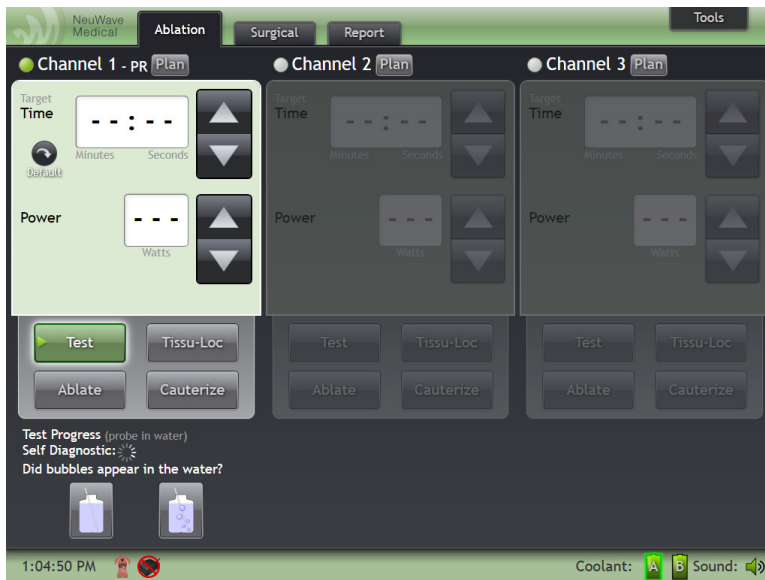
Figure 4-9: Probe on Channel 1 is being tested (Ablation Tab).
