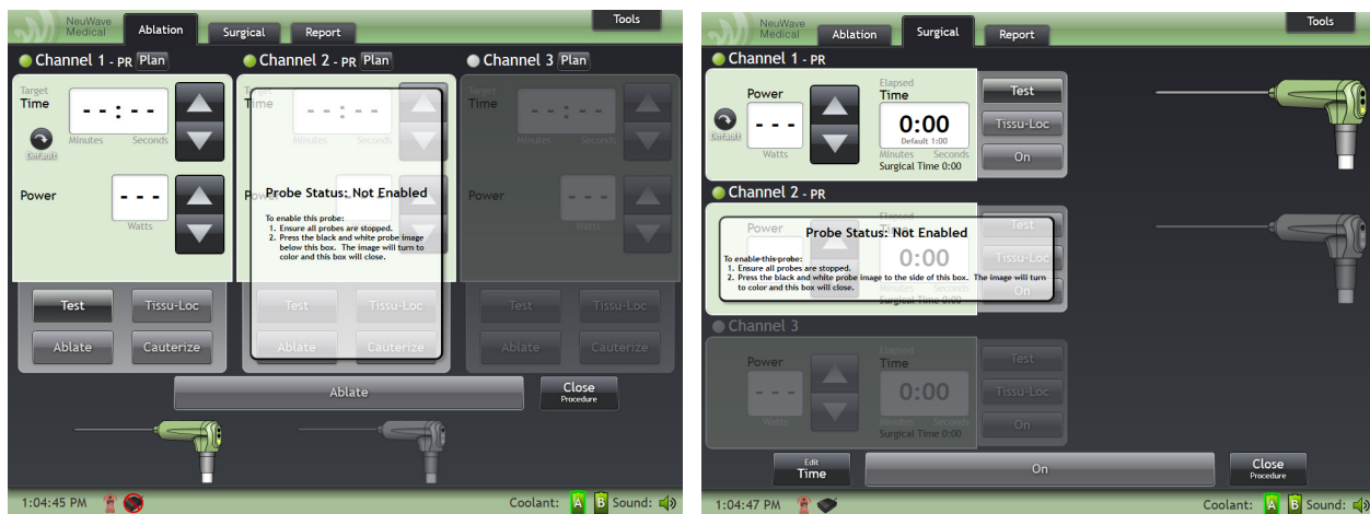
Figure 4-4: Ablation and Surgical Tab appearance when the probe connected to Channel 2 is not enabled.
