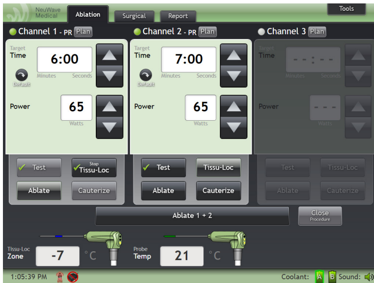
Figure 4-16: Probe connected to Channel 1 is in Tissu-Loc™ and probe connected to Channel 2 is idle.
