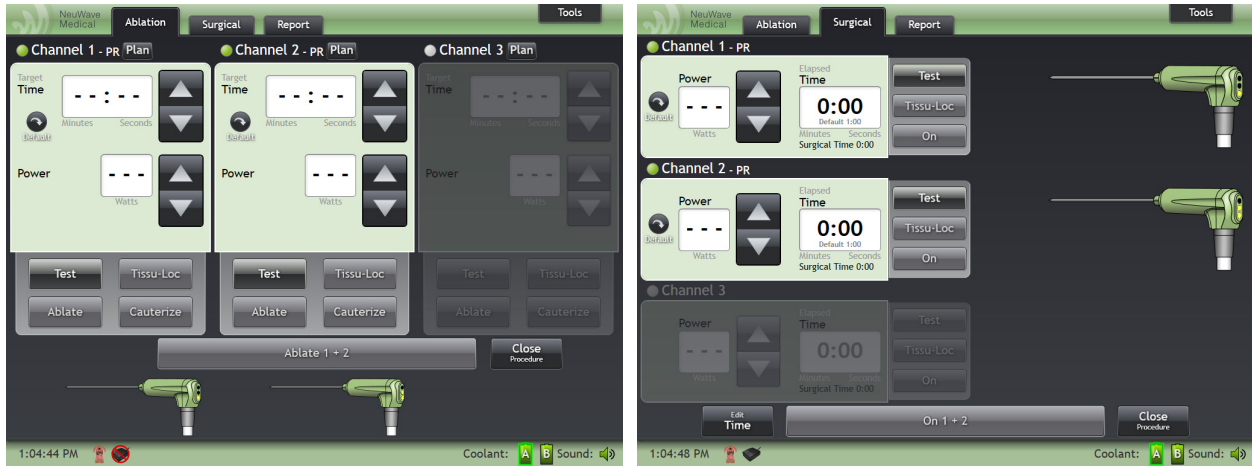
Figure 4-3: Ablation and Surgical tab appearance when multiple probes are connected. Probe images are displayed for each connected probe.
