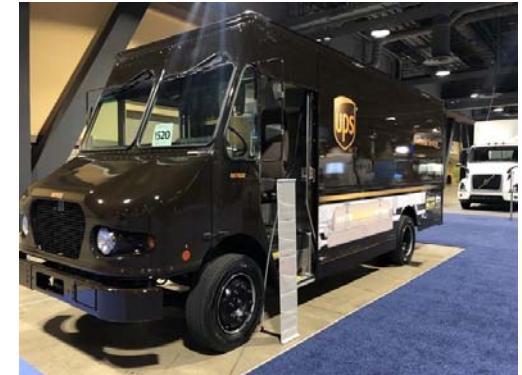
The walk-in step van manufactured by Freightliner and powered by Agility's CNG powertrain system Photo: Steven Martinez
