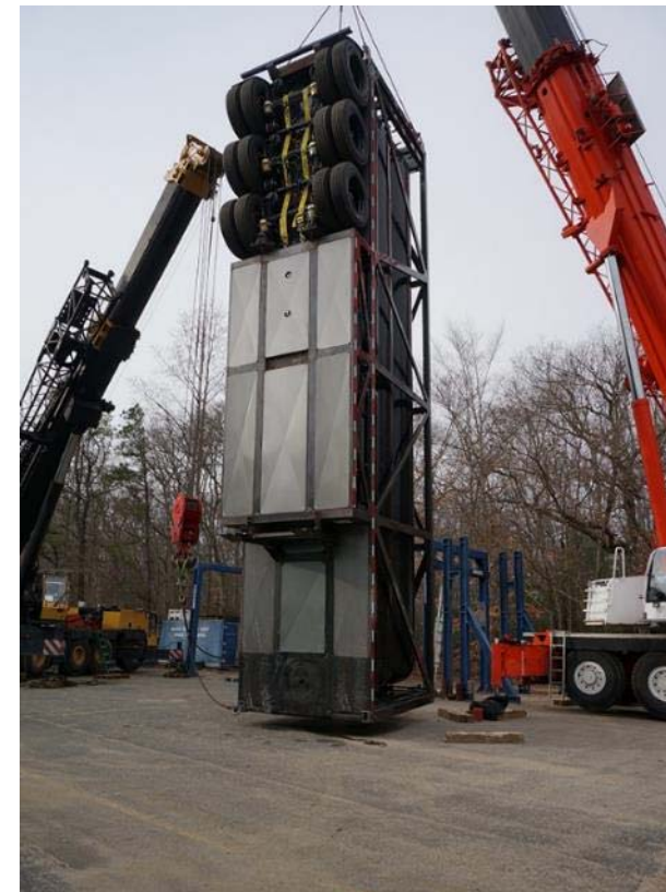
TITAN® XL passed structural container testing for US DOT application
