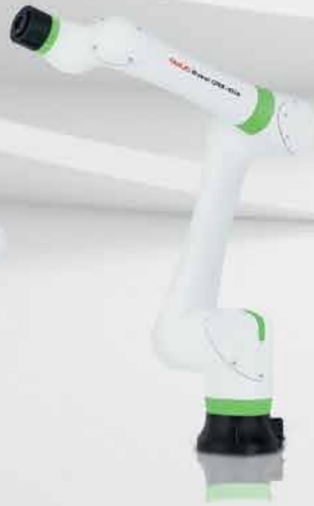
CRX-10iA Payload: 10 kg Reach: 1,249 mm
