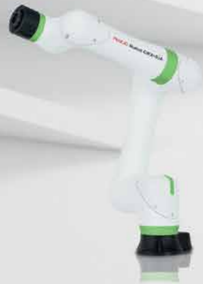
CRX-5iA Payload: 5 kg Reach: 994 mm
