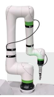
Adding to CRX Application flexibility is FANUC force sensors. A force sensor gives the robot the sense of touch and feel. This is very useful for material removal, including sanding, buffing, and deburring, as well as assembly applications. Force sensors are plug and play with FANUC's cobots including the CRX.
