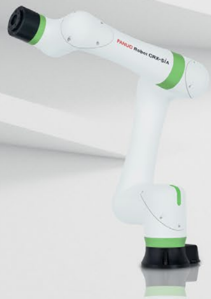
CRX-5iA Payload: 5 kg Reach: 994 mm
