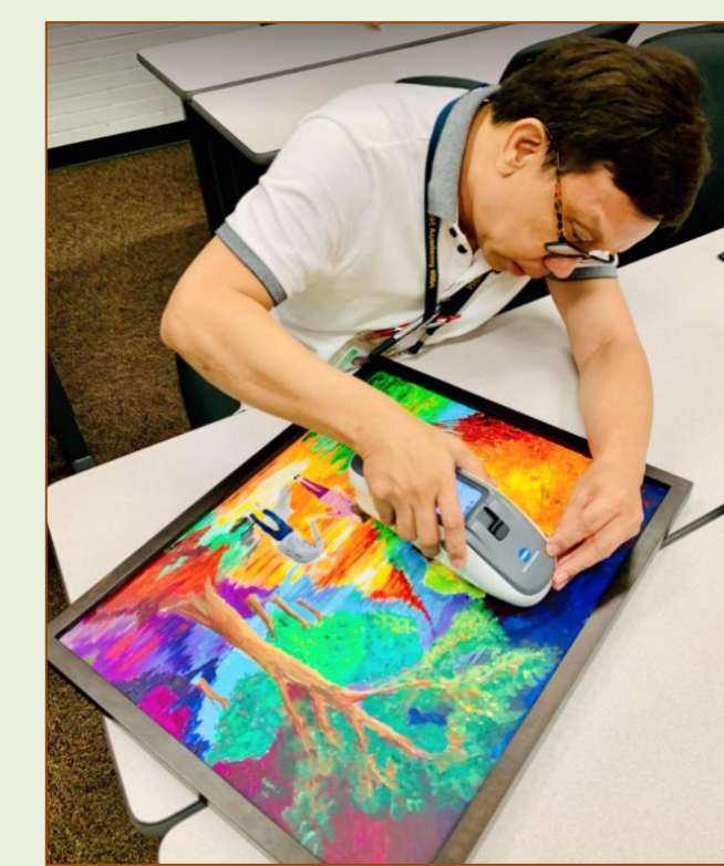
Measuring Light Absorption using Spectrophotometer
