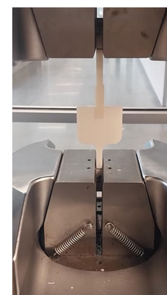
Figure 4: Servohydraulic Testing Machine Setup
