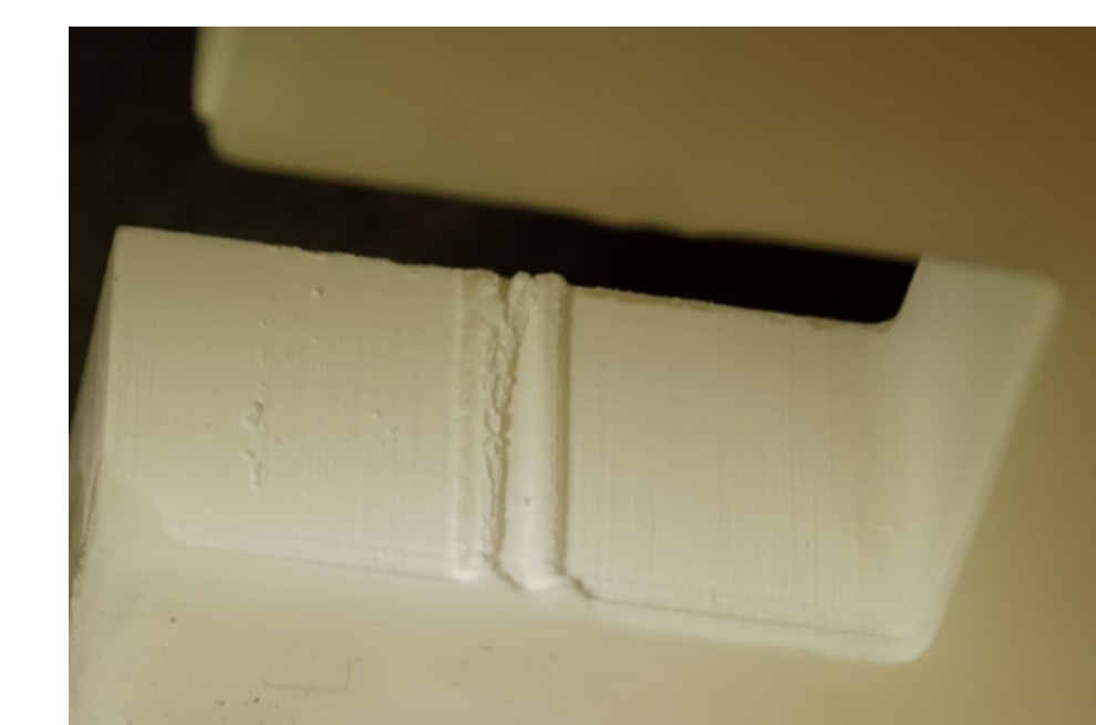
Figure 6: Shear Fracture along surface features in a successful test
