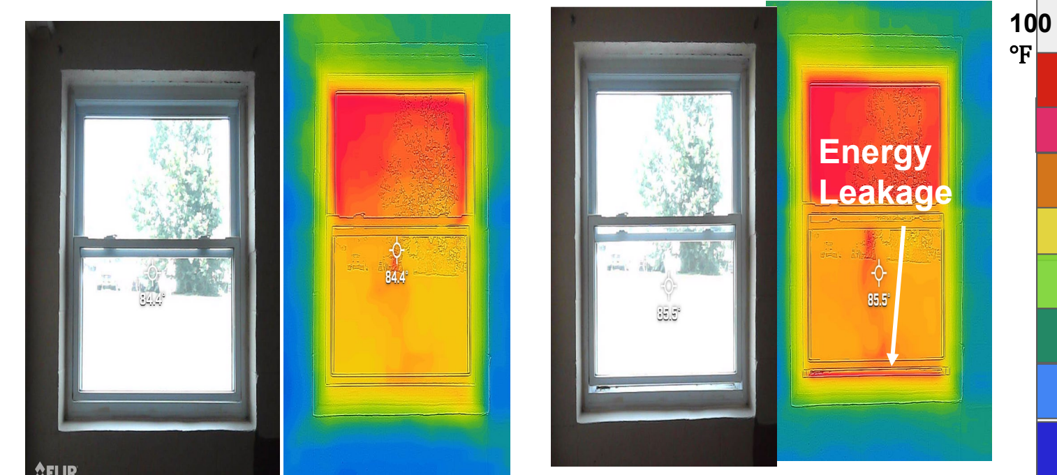
The same window gradually opened from left to right show increasing energy leakage.
