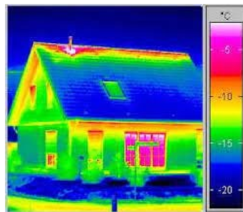
Thermal or infrared imaging interprets heat and interprets varying temperatures as color.
