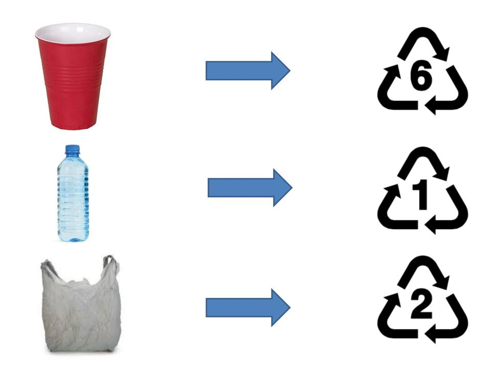
Plastic products are categorized into seven different groups which are used in sorting plastics during recycling and can help people determine how to dispose of their plastic waste.
