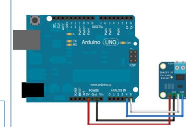
The next step in the development of this device is establishing a means of collecting highfrequency current measurement using a current sensor breakout such as the Adafruit INA219. This will allow for further development of a
