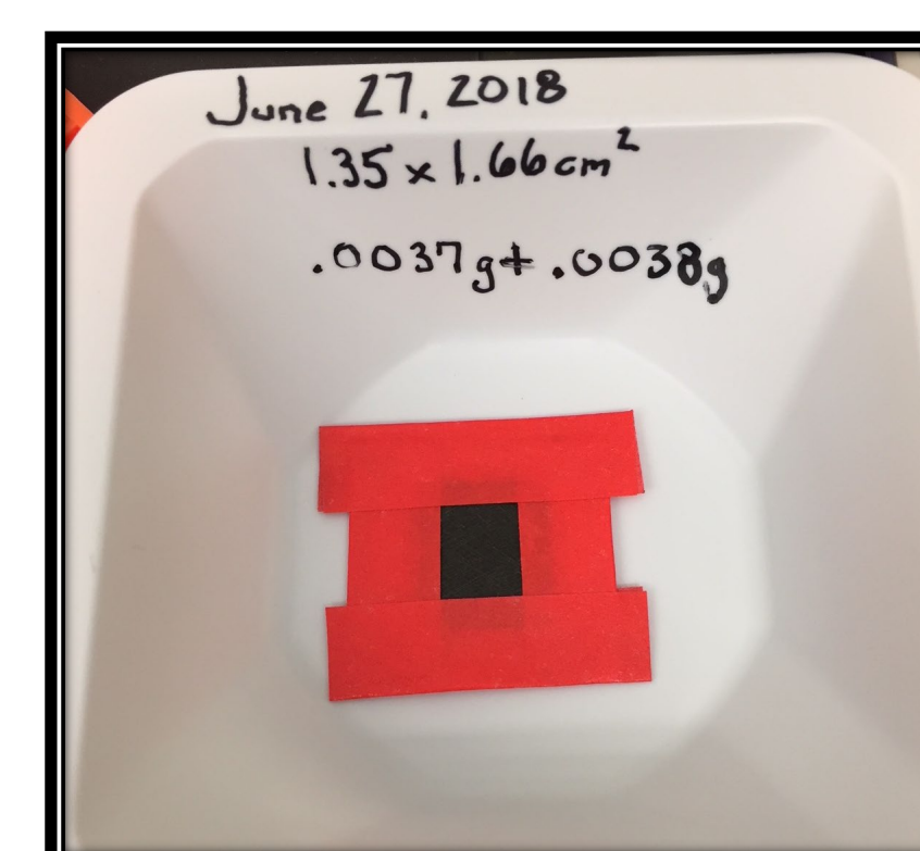
Figure 4 Left: a piece of PVA membrane that was just cast and will need to set and dry Right: A sample pseudocapacitor
