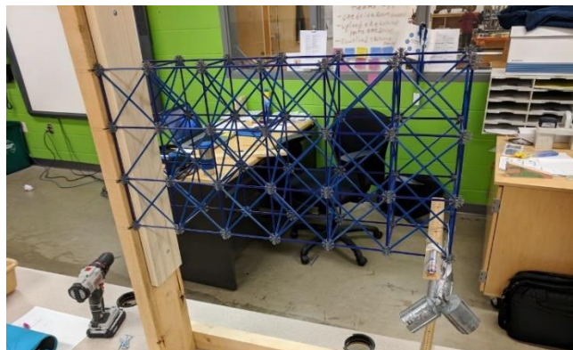
Figure 1 - A photo of the ground structure attached to the base with a 1.5 kg load applied at a distance of 24 inches from the base
